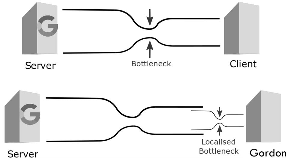
Most network dynamics, like change in bottleneck bandwidth and packet losses happen at the connection bottleneck. Localizing the bottleneck allows us to have better control over the connection.
