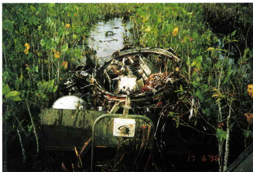
Figure 2. Remains of one of the four Cluster spacecraft in the swamps of Kourou
