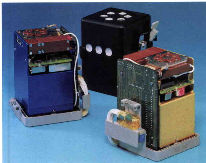
Figure 6. The space Bioreactor flown twice on the Space Shuttle (courtesy of Mécanex, IMT and the ETH Space Biology Group)
