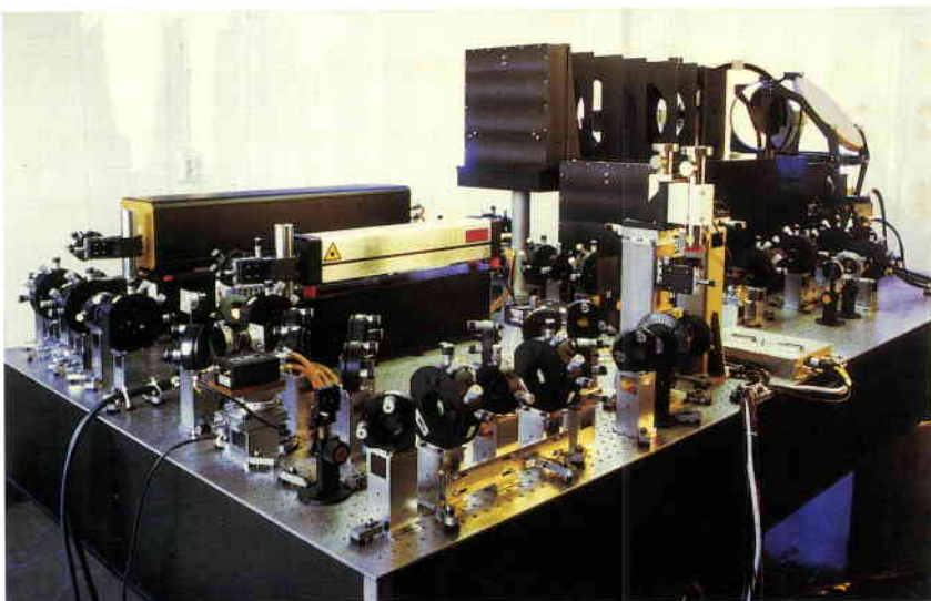
Figure 1. Laboratory breadboard model of CO 2 laser transceiver system
