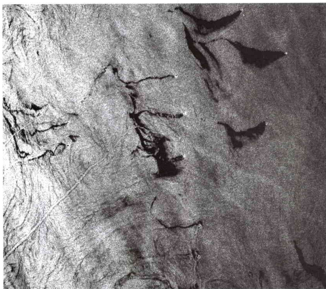
Figure 7. ERS-1 image of the Viking Bank in the North Sea acquired on 10 August 1995. It is a section of a low-resolution (100 m) image produced for near real-time delivery to the pollution control authorities. The bright points in the image are oil rigs. The black areas emanating from them are probably waste water or drilling fluid (courtesy of TSS and ESRIN)
