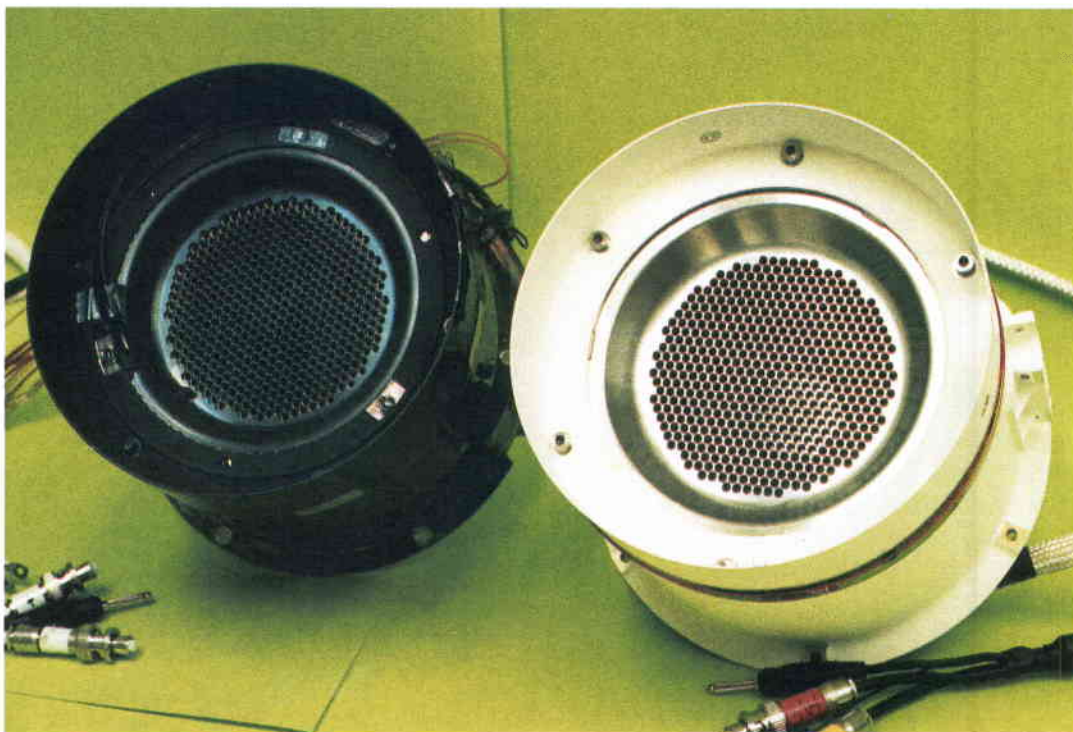
Figure 5: Engineering model of the Radio Frequency Ion Thruster, courtesy of DASA
