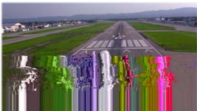
The effect of jitter and lost packets on the video quality
