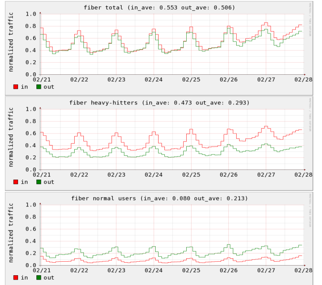
Figure 18: Fiber weekly traffic: total fiber users (top), heavy-hitters (middle) and normal users (bottom)
