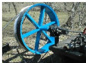
Figure 80: Cable guide pulley
