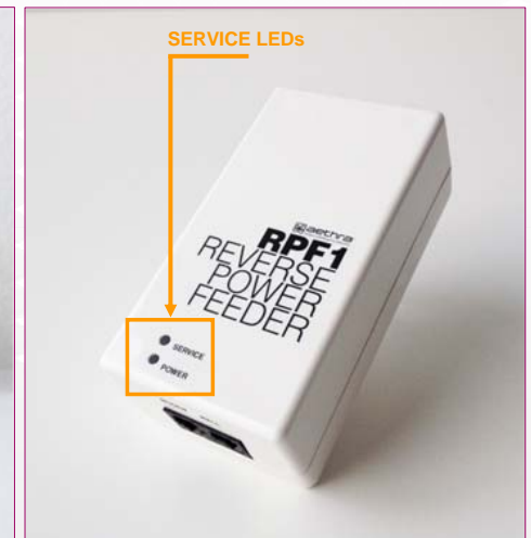
Figure 2: RPF connectors and LEDs
