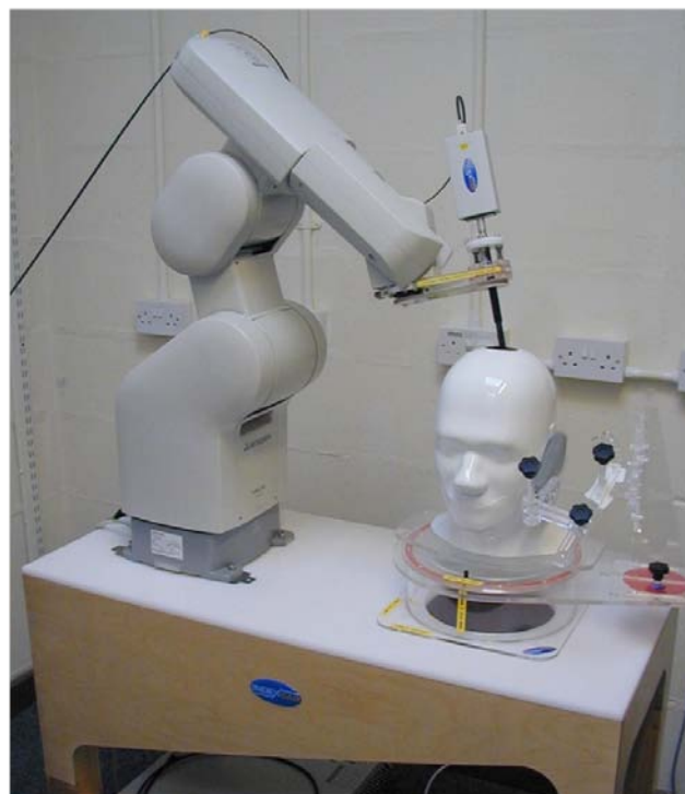
Head phantom and robotic arm used to make specific energy absorption rate (SAR) measurements
