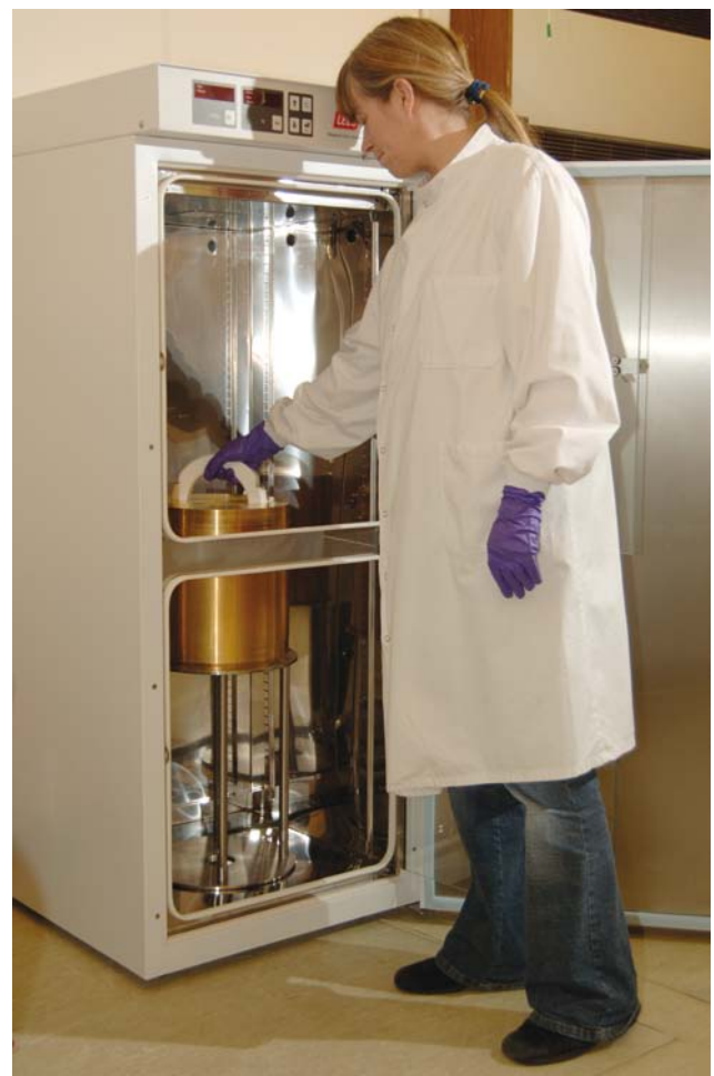
Loading the doubly resonant cavity in preparation for an exposure (photograph courtesy of Public Health England)
