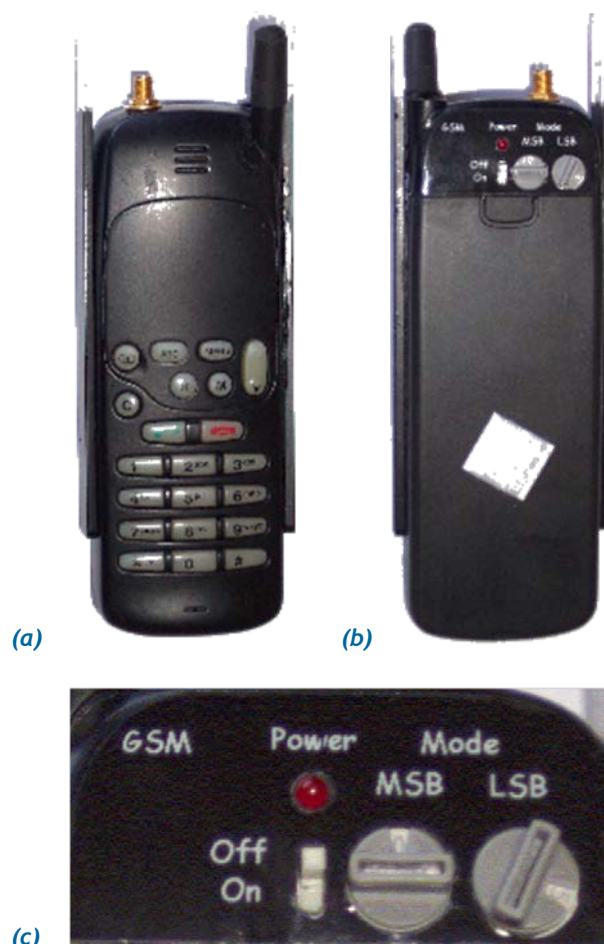
FIGURE A1 (a) front, (b) back and (c) control switches of the GSM phone exposure system
