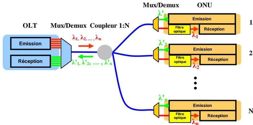
Figure 2—5 : Architecture PON WDM bidirectionnelle "broadcast and select"
