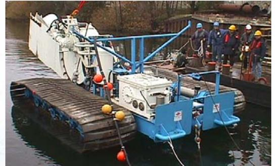
*...using TM02 trencher equipped with cutting wheel*
