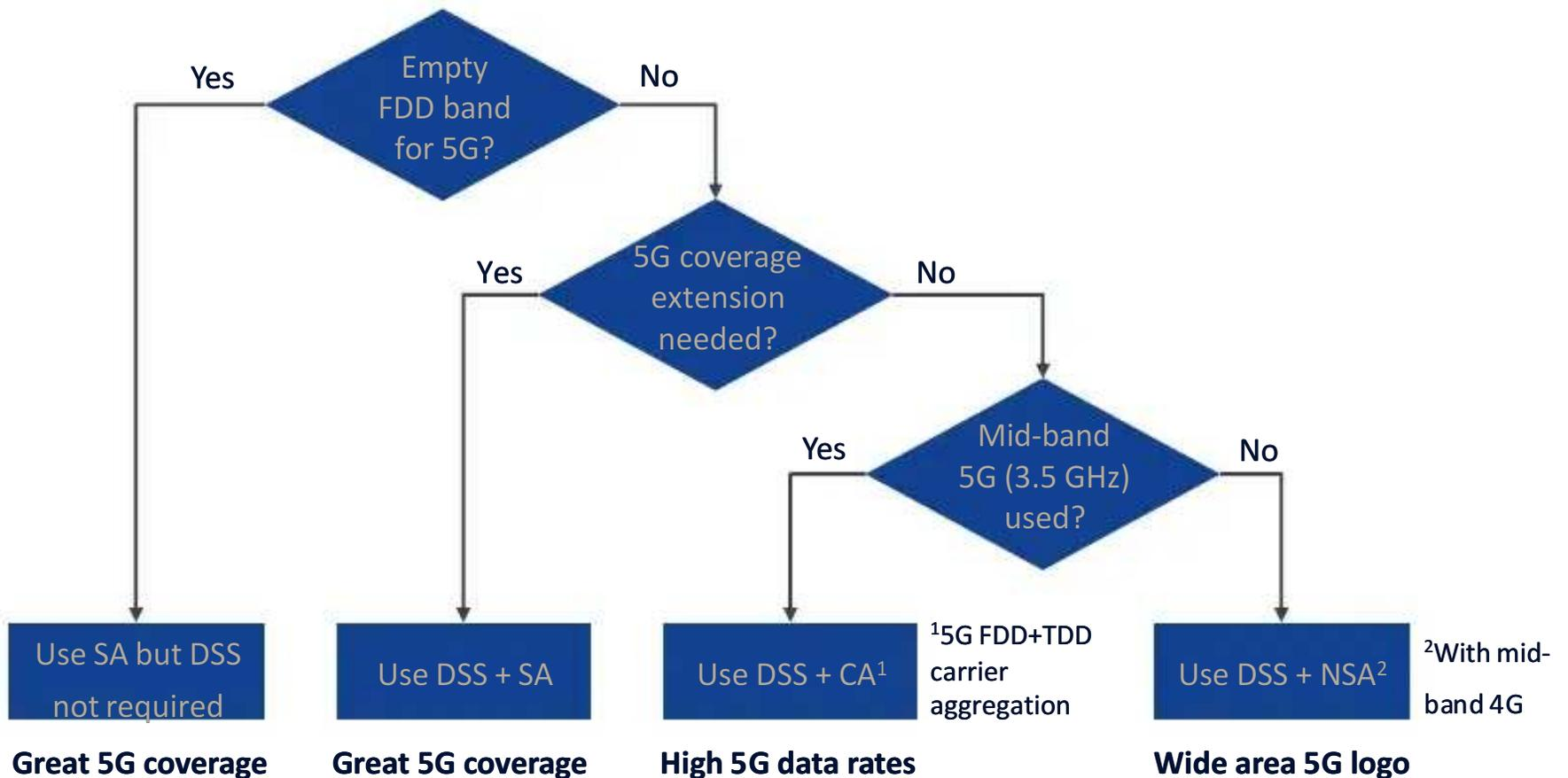
Figure 5. DSS with 5G core network and 5G carrier aggregation delivers the optimum set of 5G benefits
