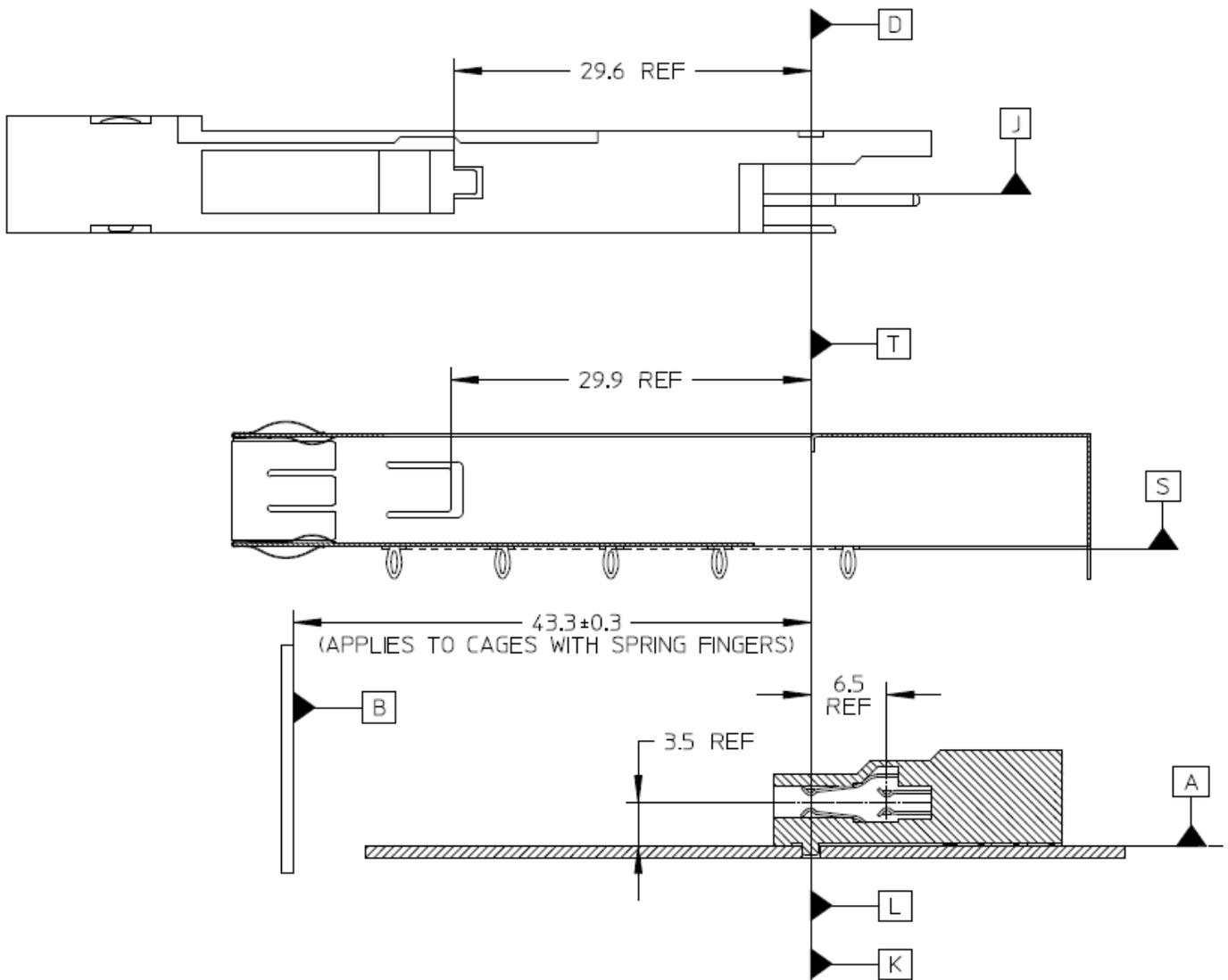
**Figure 14: Surface mount connector/cage datum descriptions**
