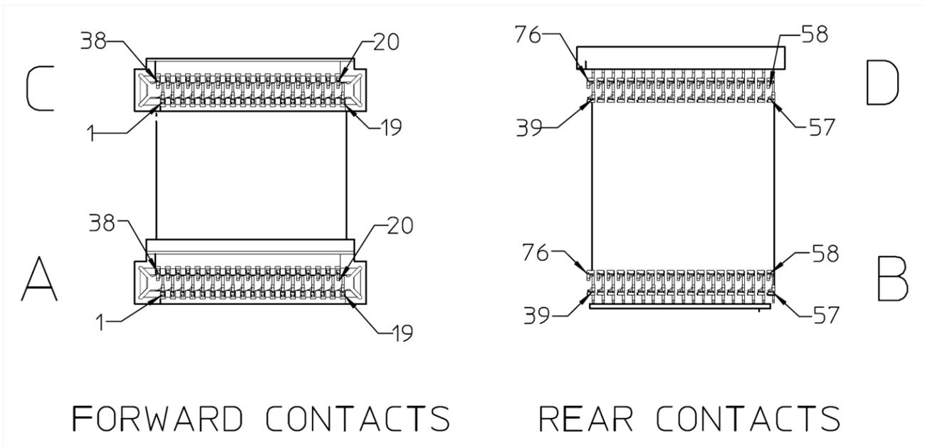
Figure 26: Connector pins in 2x1 stacked cage as viewed from the front
