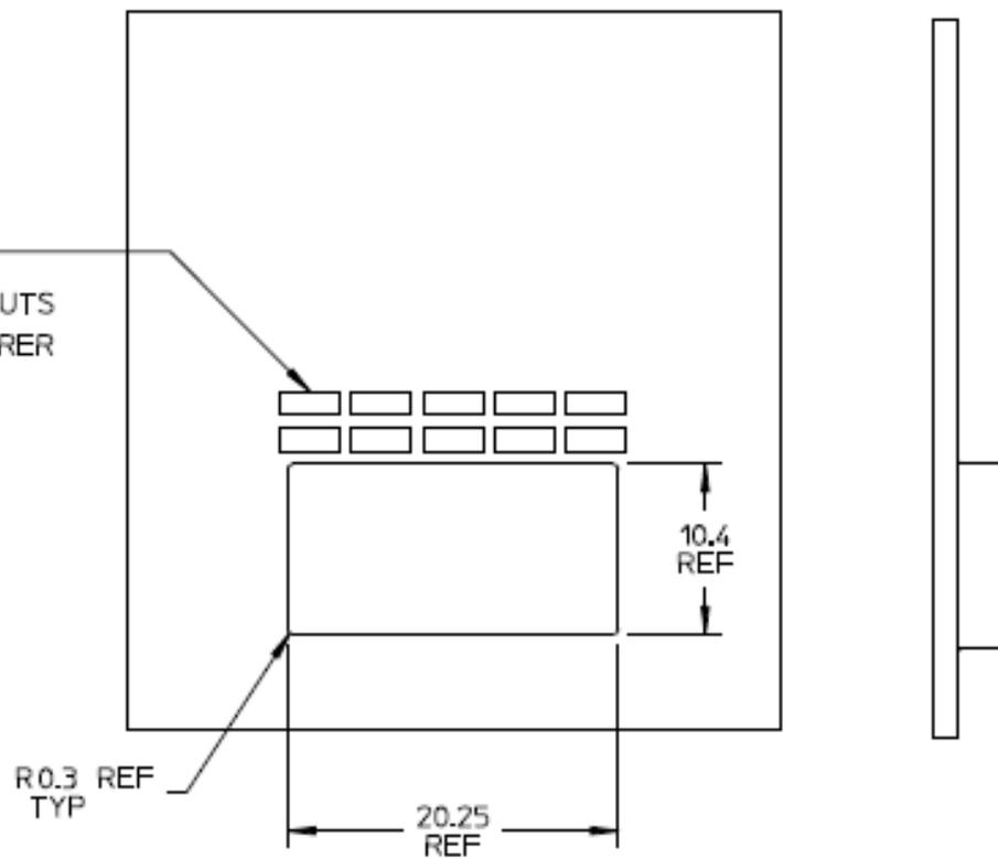
Figure B-2: Type 2A example 1X1 bezel design
