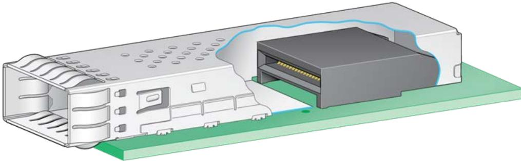
**Figure 30: SMT connector in 1xn cage**
