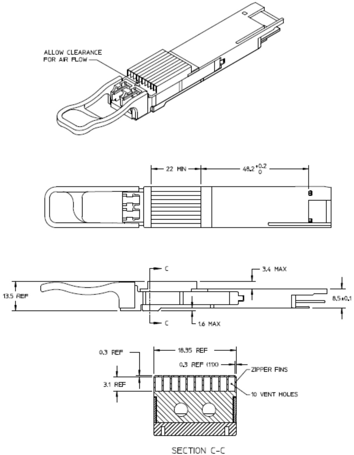
Figure B-6: Type 2A Zipper Fin Heat Sink Example
