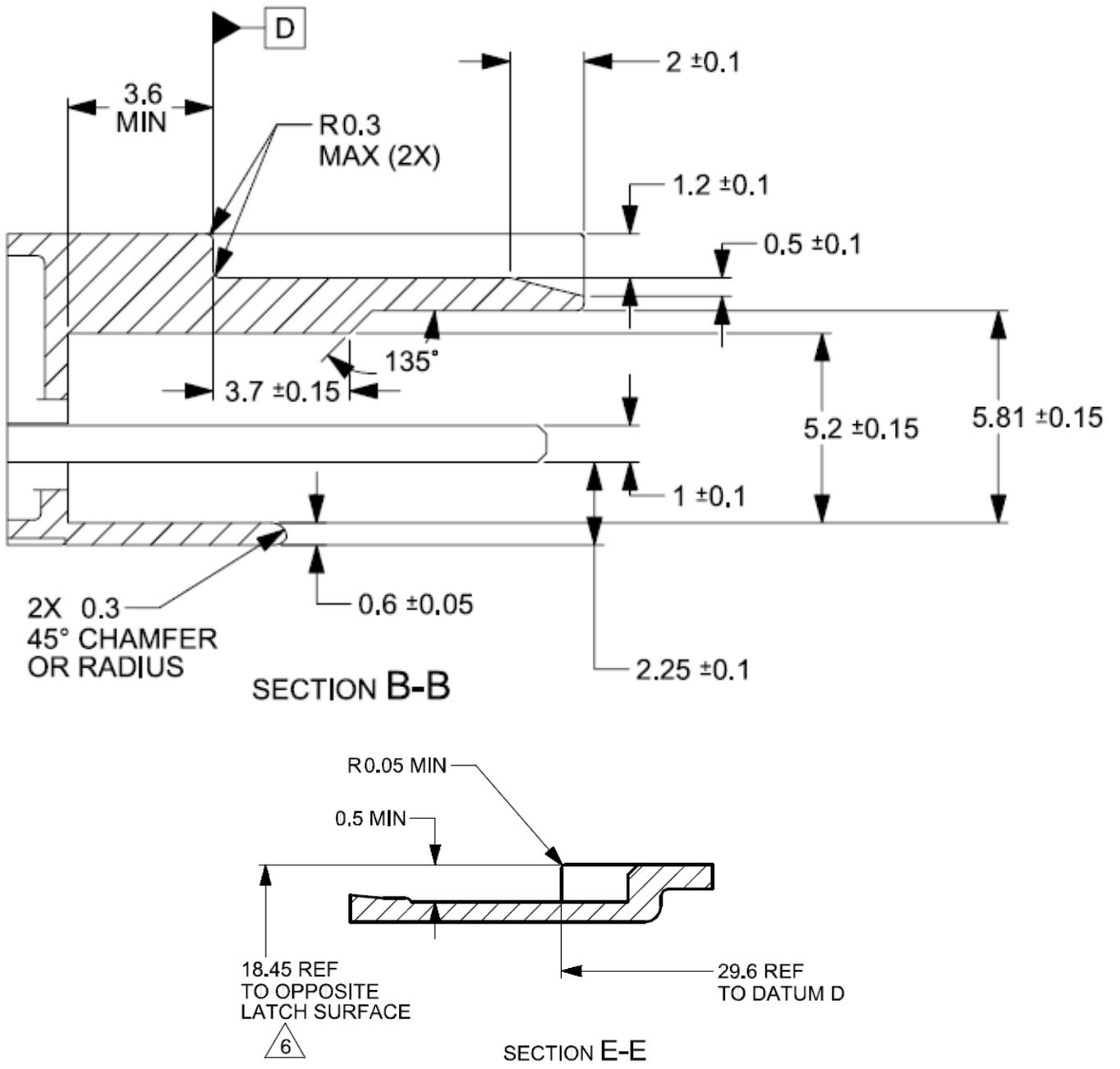
Figure 20: Detailed dimensions of module
