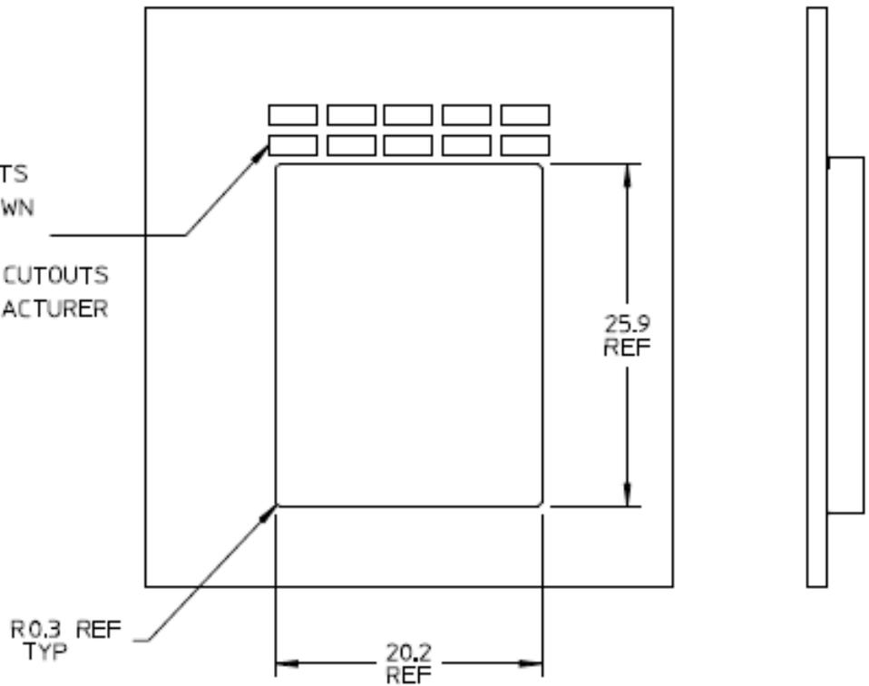
Figure B-3: Type 2A example 2X1 bezel design
