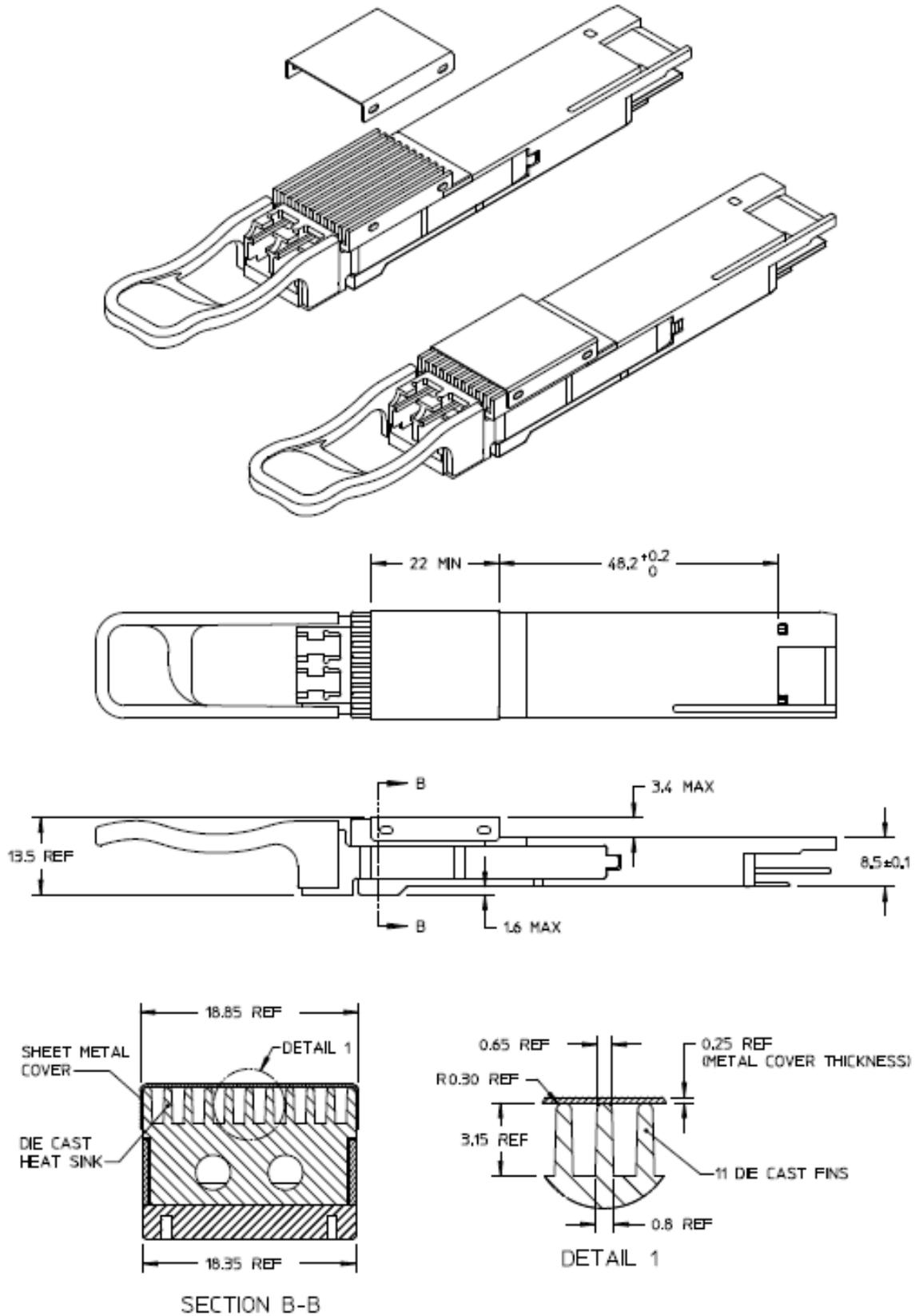
Figure B-5: Type 2A Die Cast Heat Sink with Metal Cover Example
