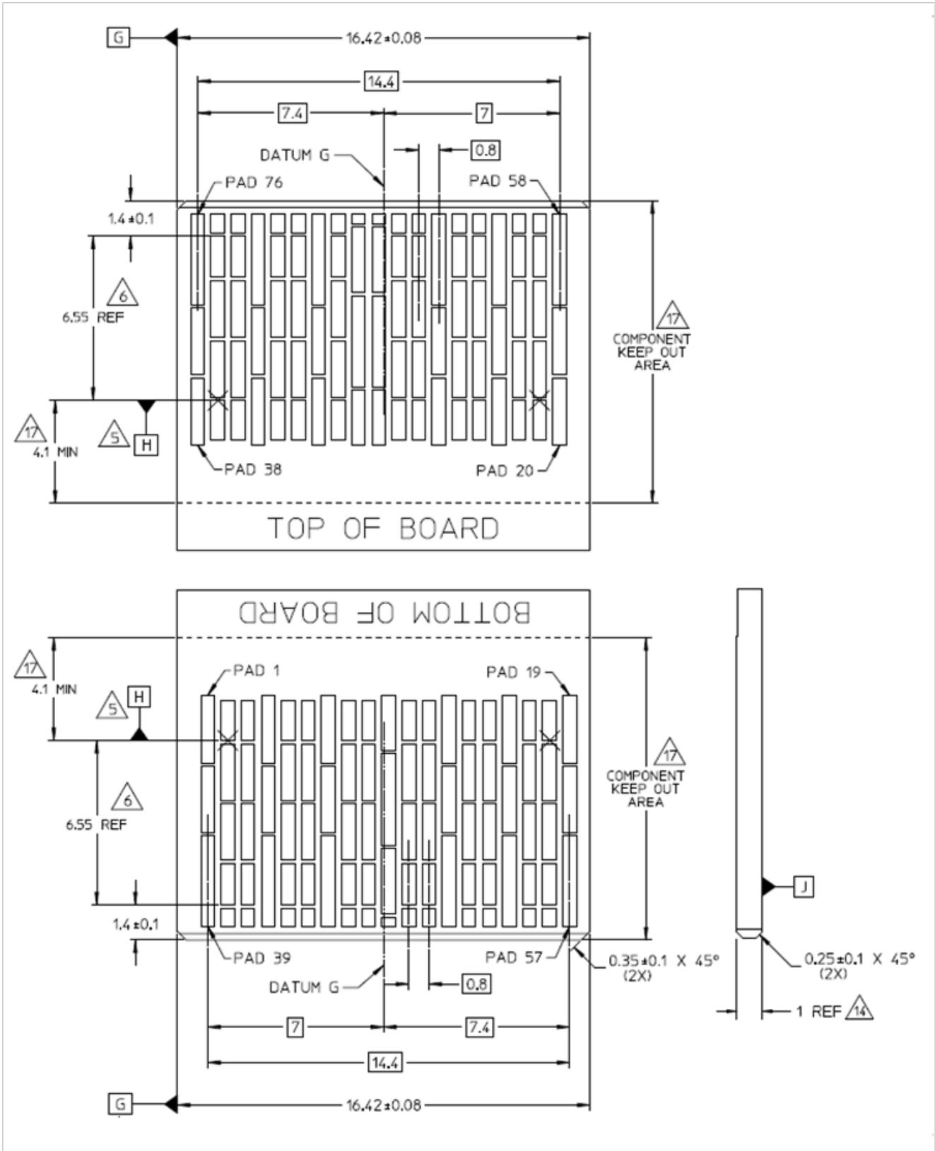
Figure 21: Module paddle card dimensions
