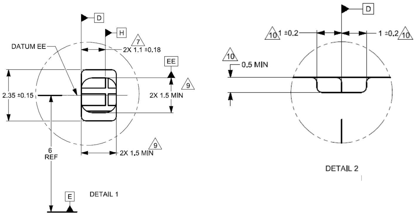
Figure 18: Drawing of module
