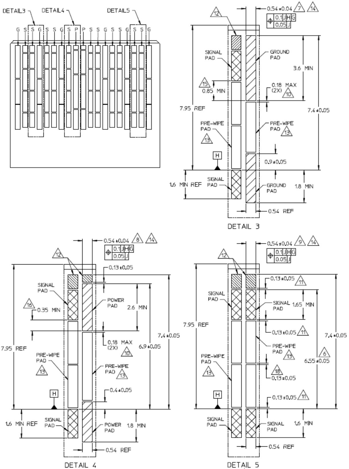
Figure 22: Module pad dimensions
