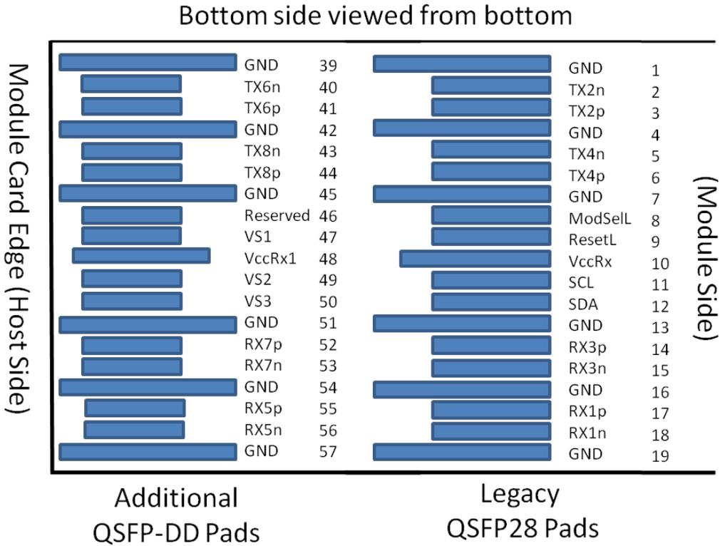
Figure 2: Module pad layout
