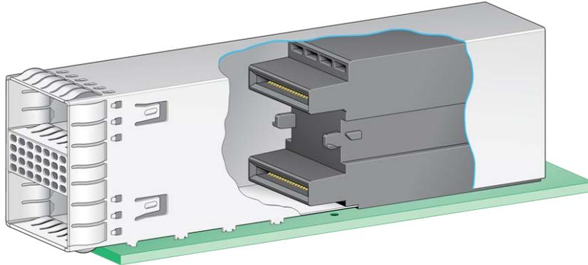
**Figure 23: Integrated connector in 2x1 stacked cage**
