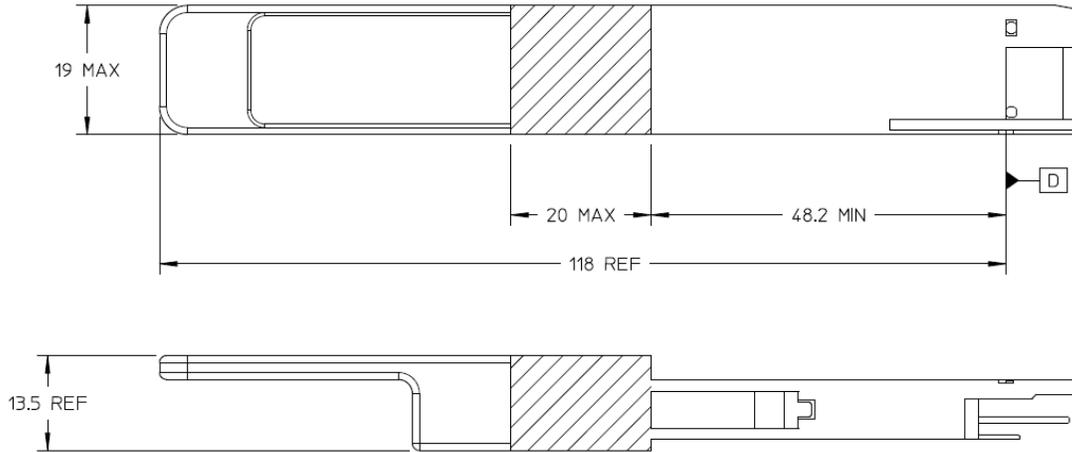
**Figure 46: Informative overall module length with handle for Type 1 module**
