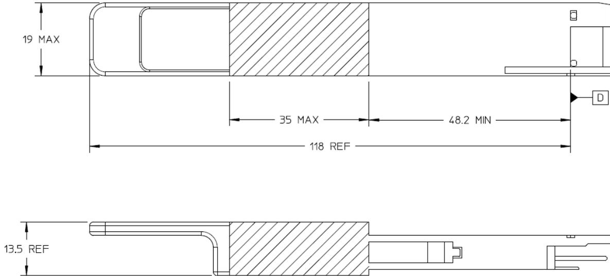
**Figure 47: Informative overall module length with handle for Type 2 and Type 2A modules**
