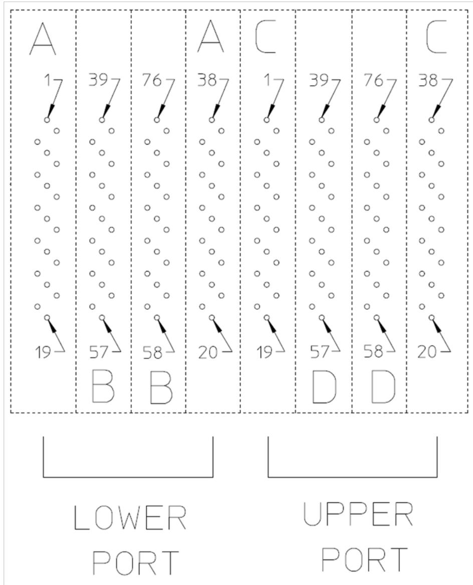
**Figure 28: 2X1 host board connector contacts**
