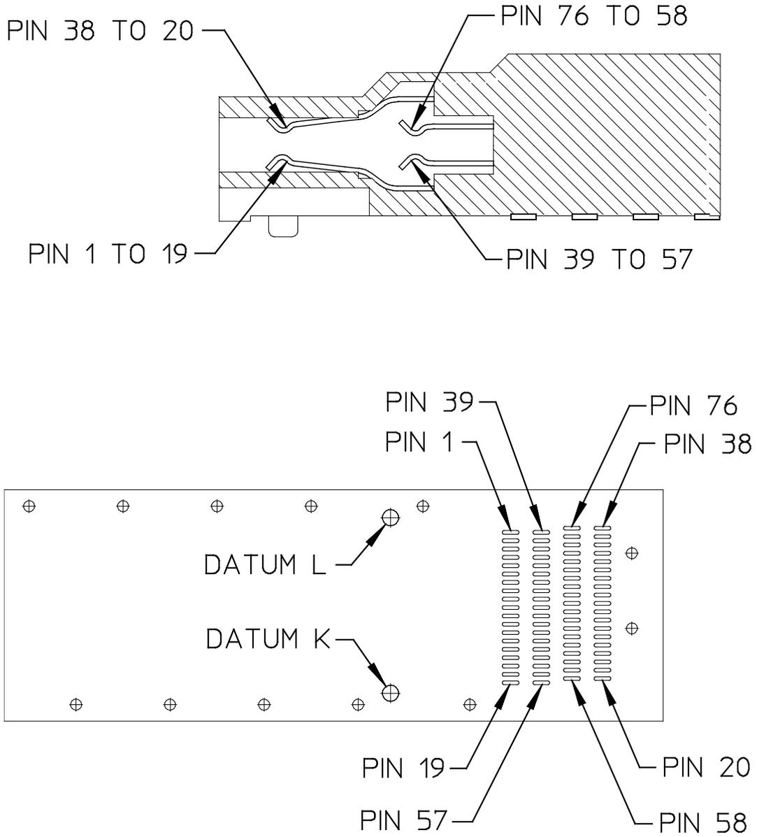
Figure 35: SMT Connector and Host PCB Pin Numbers
