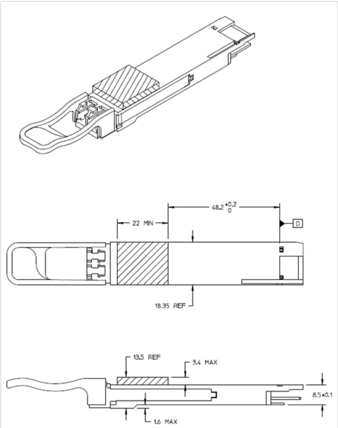
Figure 19: Type 2A Module with Heat Sink
