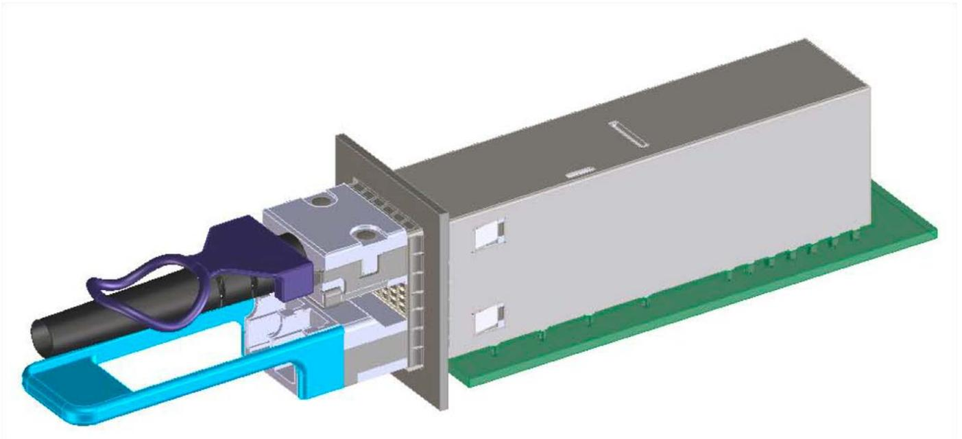
Figure 9: 2x1 stacked cage and module
