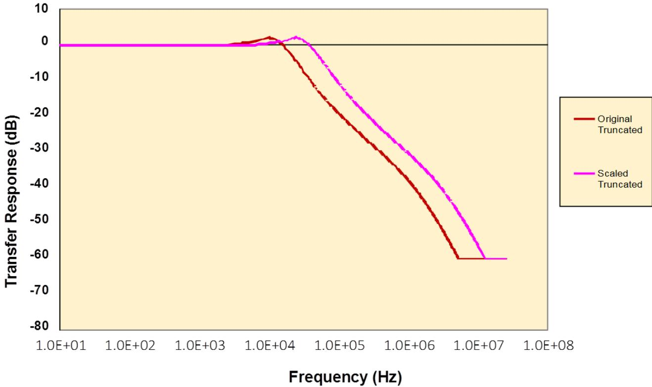
**Figure 8: Truncated Transfer Response for Host Board Power Supply Noise Output measurement**
