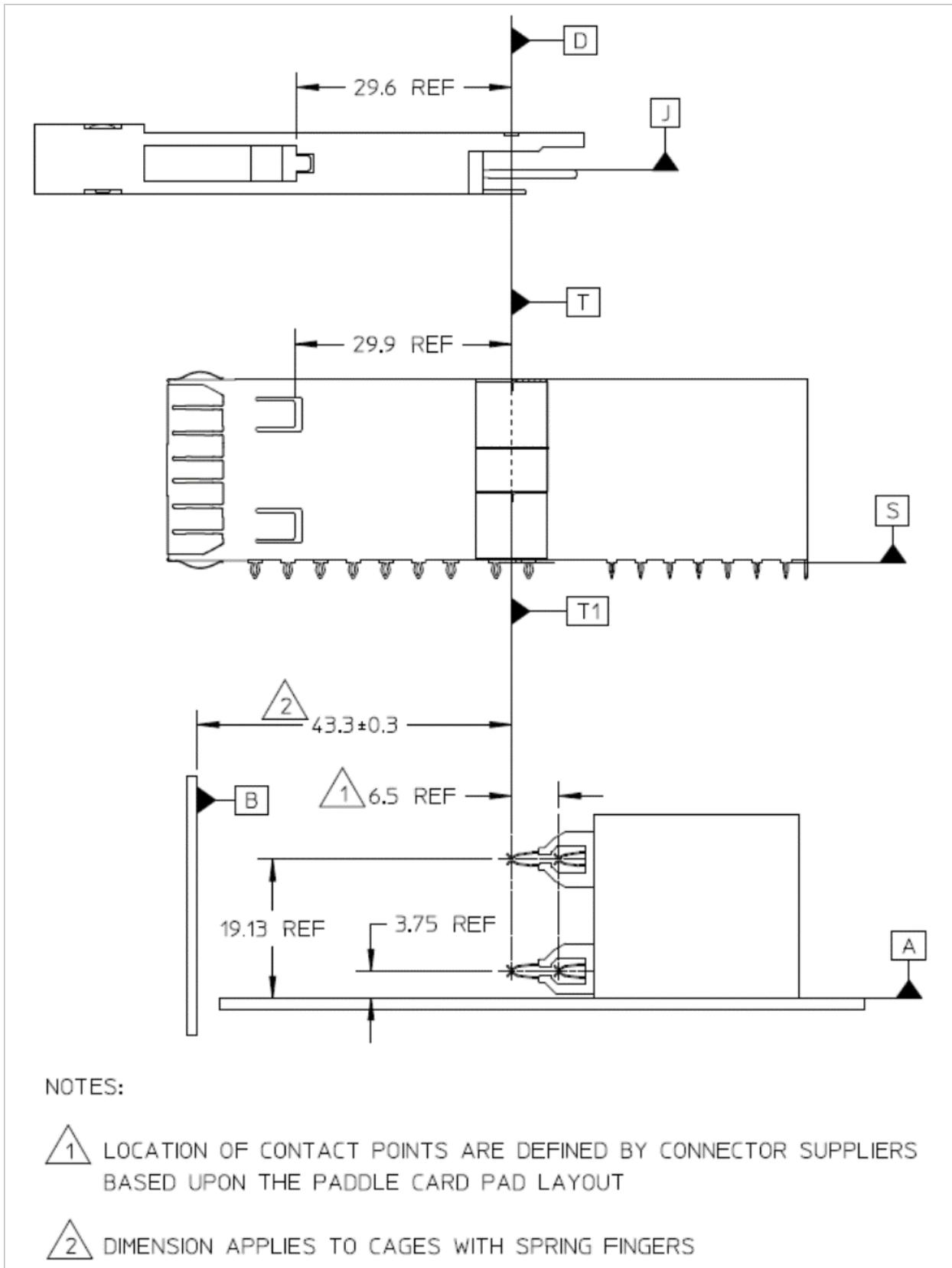
Figure 13: 2X1 stacked connector/cage datum descriptions
