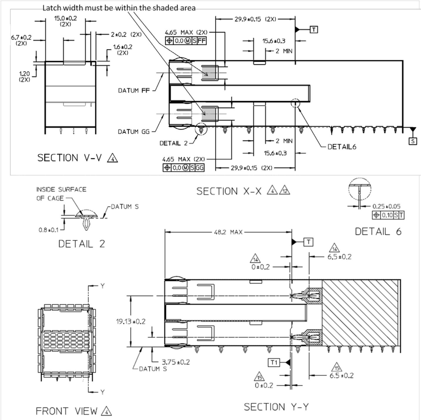
Figure 25: 2x1 stacked cage dimensions
