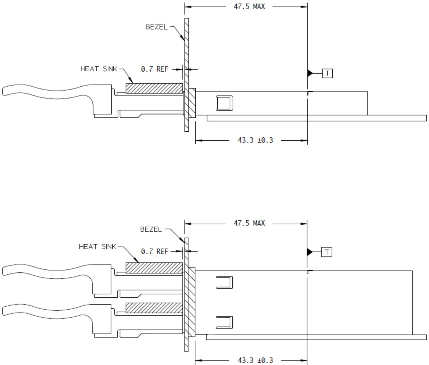
Figure B-1: Type 2A example module insertion
