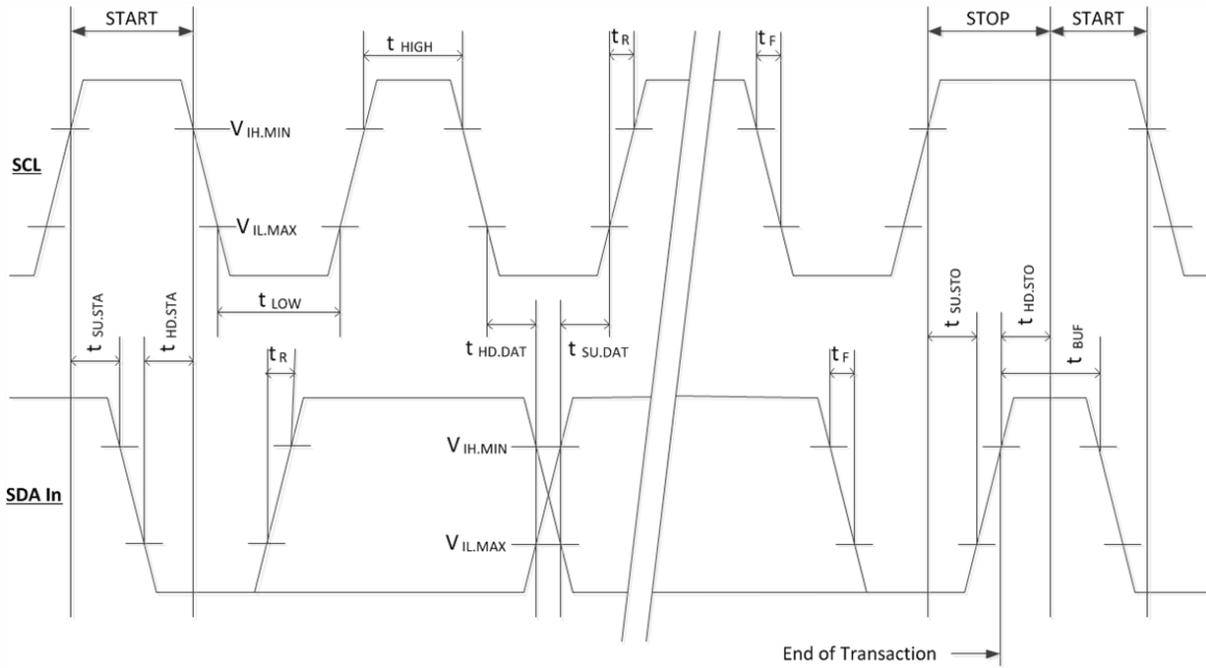
Figure 44: QSFP-DD Timing Diagram
