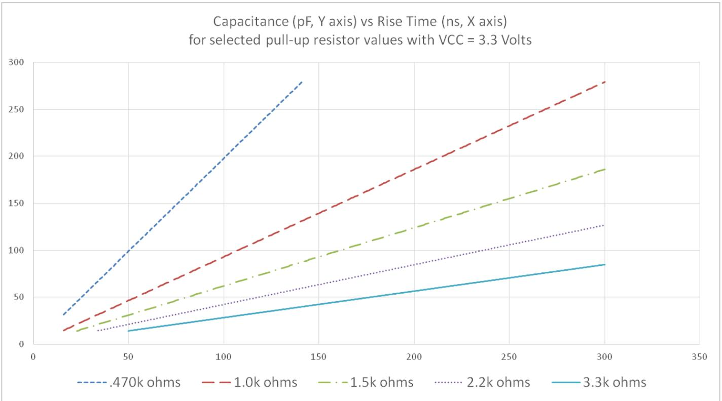
**Figure 45: SDA/SCL options for pull-up resistor, bus capacitance and rise/fall times**
